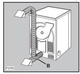
Once connected to the dryer, run the vent hose to the desired outlet point, ensuring that the run's overall length is less than 2.5 m, and that it contains no more than two bends. As to the outlet itself, if you have decided on a fixed wall/window grille, a good local builder's merchant should be able to supply you with the necessary fittings and installation advice.
